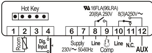
NOTE: The compressor relay is 20(8)A or 16(6)A depending on the model.
