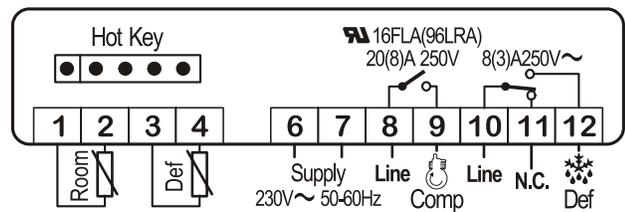
NOTE: The compressor relay is 20(8)A or 16(6)A depending on the model.
