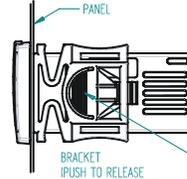
Instrument XR03CX and XR04CX shall be mounted on vertical panel, in a 29x71 mm hole, and fixed using the special bracket supplied.
